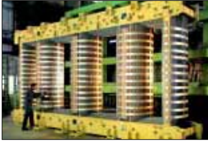
Core assembly of 250MVA Generator Transformer
