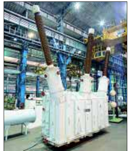
63 MVAR, 420kV Reactor
